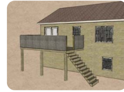
Uncovered deck greater than 0.6 m in height
