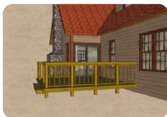
(2) uncovered decks less than 0.6 m in height do not require a permit
